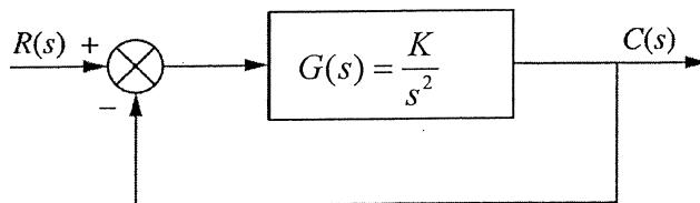
is to be designed for a settling time of 1.667 seconds and a 16.3% overshoot. If a compensator zero is placed at -1, do the following:
