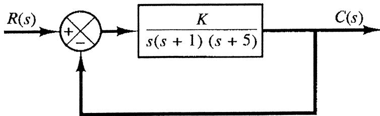
after normalizing the given transfer function. You need to sketch magnitude and phase plots for each component first (i.e., overall gain after normalization, and three poles). Then you need to show the overall Bode diagram.
